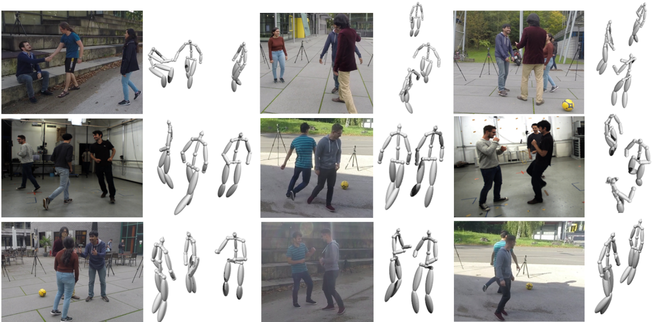
Figure 3. Visualization of our results on MuPoTS-3D Test Set from different viewpoints. Notice that the model is fairly robust to occlusions. The spatial alignment is not derived from ground truth.
