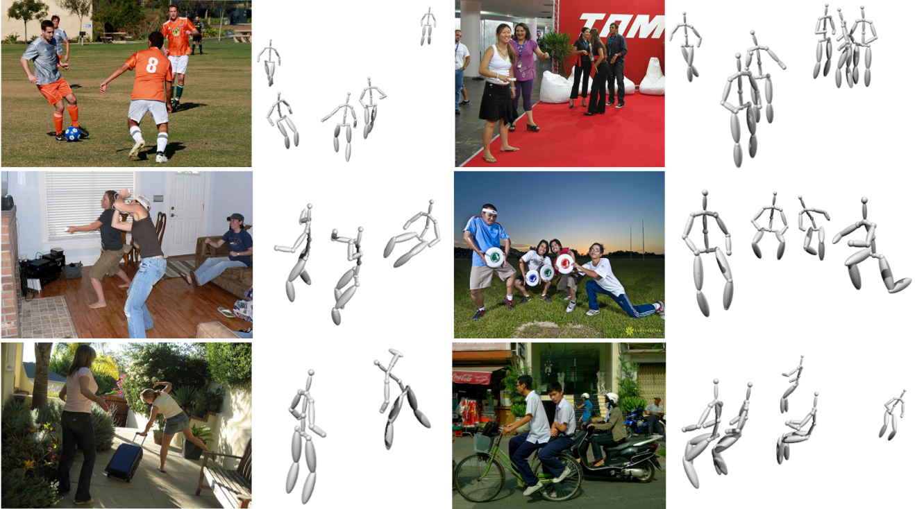
Figure 1. Some results of our proposed 3D pose estimation pipeline on some challenging samples from MS COCO. Our approach is resilient against occlusions and clutter. We also approximate the spatial ordering of people in the scene with respect to the camera. Further in-the-wild results and a 3D rendered view of the above images can be found in the supplementary material.
