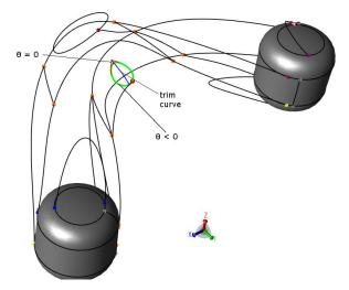
Figure: Example of a non-decomposable sweep: a cylinder being swept along a cosine curve in *xy*-plane while undergoing rotation about *x*-axis. The curve  $\theta = 0$  is shown in red and trim curve is shown in blue. The portion of the swept edges where  $\theta$  is negative is shown in green.
