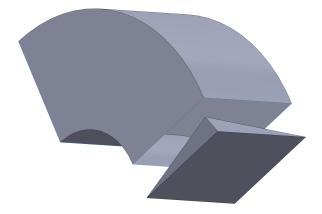
Figure: A pyramid swept along a curvilinear trajectory
