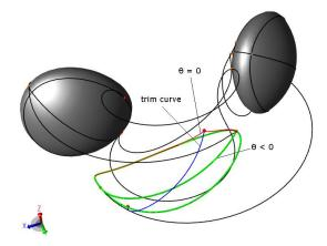
Figure: Example of a non-decomposable sweep: a blended intersection of a sphere and an ellipsoid being swept along a circular arc in *xy*-plane while undergoing rotation about *z*-axis. The curve  $\theta = 0$  is shown in red and trim curve is shown in blue. The portion of the swept edges where  $\theta$  is negative is shown in green.
