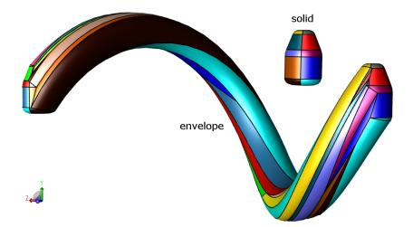
Figure: A simple bottle being swept along a screw motion with compounded rotation. Correspondence between faces of  $\partial M$  and those of the envelope is shown by color coding.
