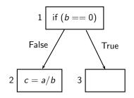
Placing a/b at the exit of 1 is unsafe  $(\equiv can change the behaviour of$ the optimized program)
