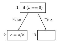
Placing a/b at the exit of 1 is unsafe ( $\equiv$  can change the behaviour of the optimized program)
