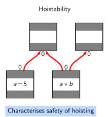
Hoist an expression to the entry of a block only if it can be hoisted out of the block into all predecessor blocks
