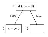
Placing a/b at the exit of 1 is unsafe ( $\equiv$  can change the behaviour of the optimized program)
