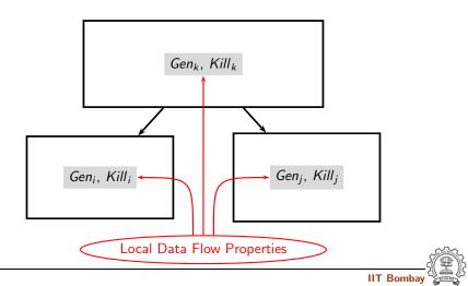
$Gen_n = \{ v \mid \text{variable } v \text{ is used in basic block } n \text{ and} \\ \text{is not preceded by a definition of } v \} \\ Kill_n = \{ v \mid \text{basic block } n \text{ contains a definition of } v \}$
