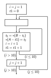
• The only activity in the outer loop now is to control the loop iterations
