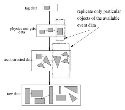
Figure 6. Replication of objects using XML in the CMS Event Data Model
