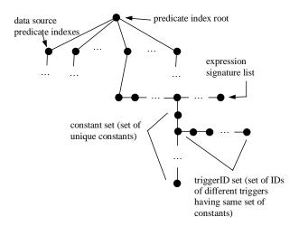
Figure 4. Expanded View of Normalized Predicate Index Structure.
