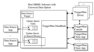
Figure 1. The architecture of the TriggerMan trigger processor.
