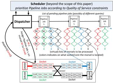
Example NUMA Multi-Core Server with 4 Sockets and 32 Cores
