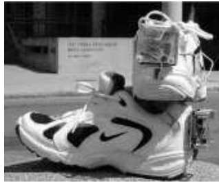
Figure 10: Functional prototype of piezoelectric-powered RFID shoes with mounted electronics.
