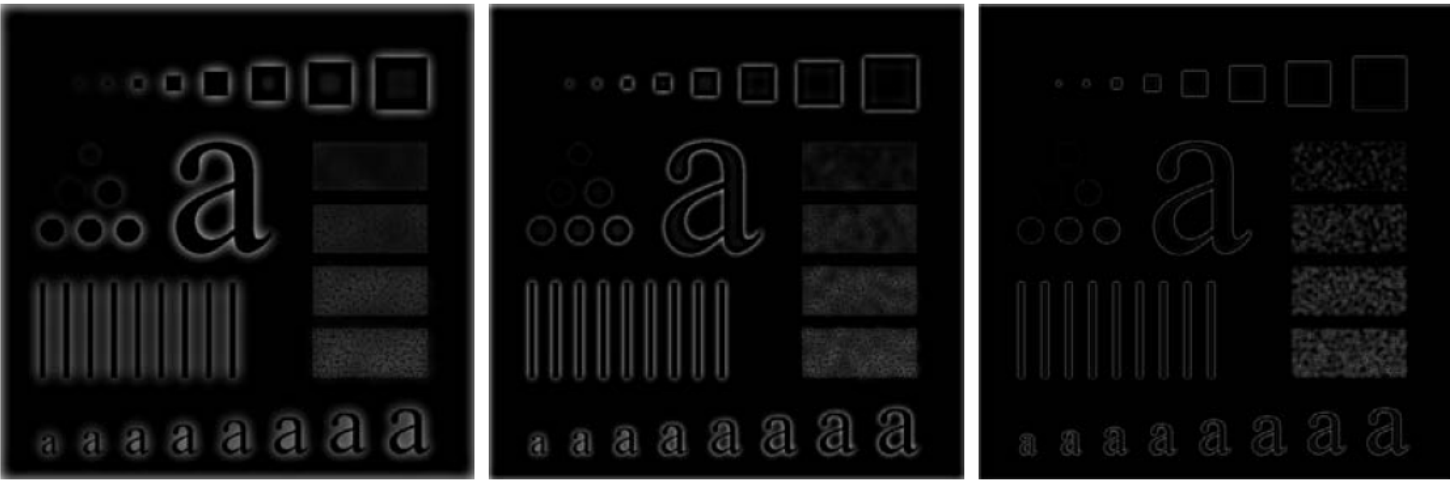
FIGURE 4.54 Results of highpass filtering the image in Fig. 4.41(a) using an IHPF with D_0 = 30, 60, and 160.
