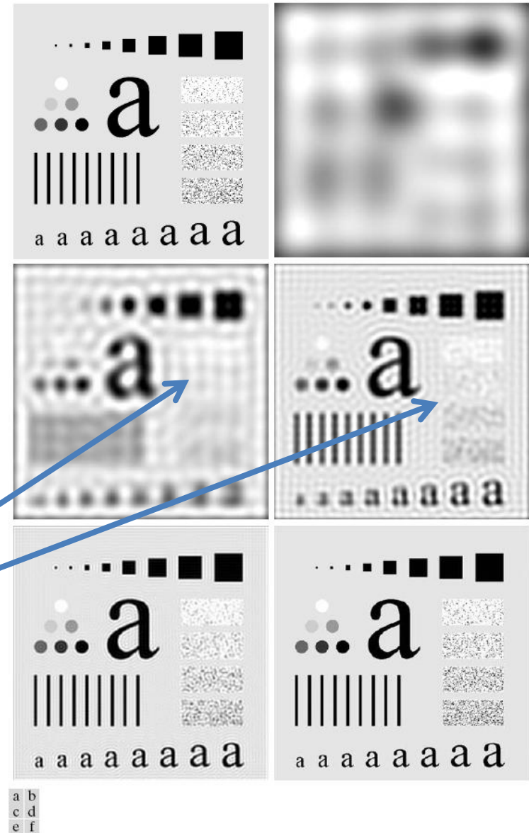
FIGURE 4.42 (a) Original image. (b)–(f) Results of filtering using ILPFs with cutoff frequencies set at radii values 10, 30, 60, 160, and 460, as shown in Fig. 4.41(b). The power removed by these filters was 13, 6.9, 4.3, 2.2, and 0.8% of the total, respectively.
