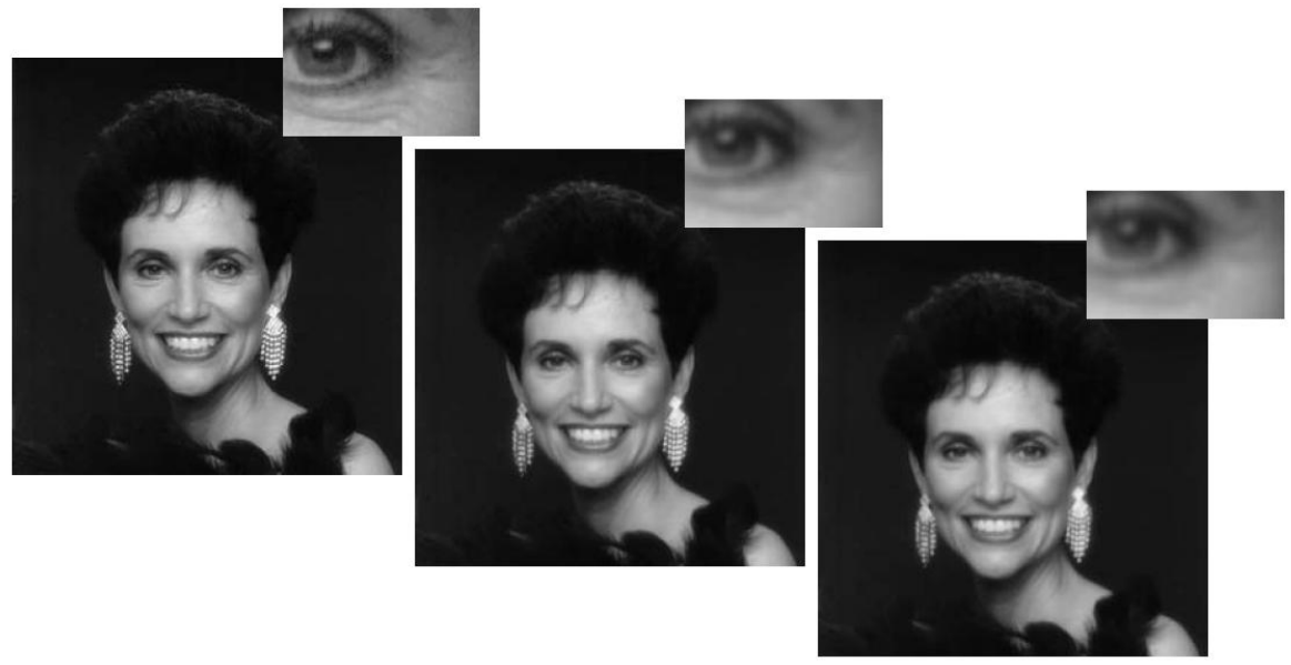
FIGURE 4.50 (a) Original image ( 784 \times 732 pixels). (b) Result of filtering using a GLPF with D_0 = 100 . (c) Result of filtering using a GLPF with D_0 = 80 . Note the reduction in fine skin lines in the magnified sections in (b) and (c).
