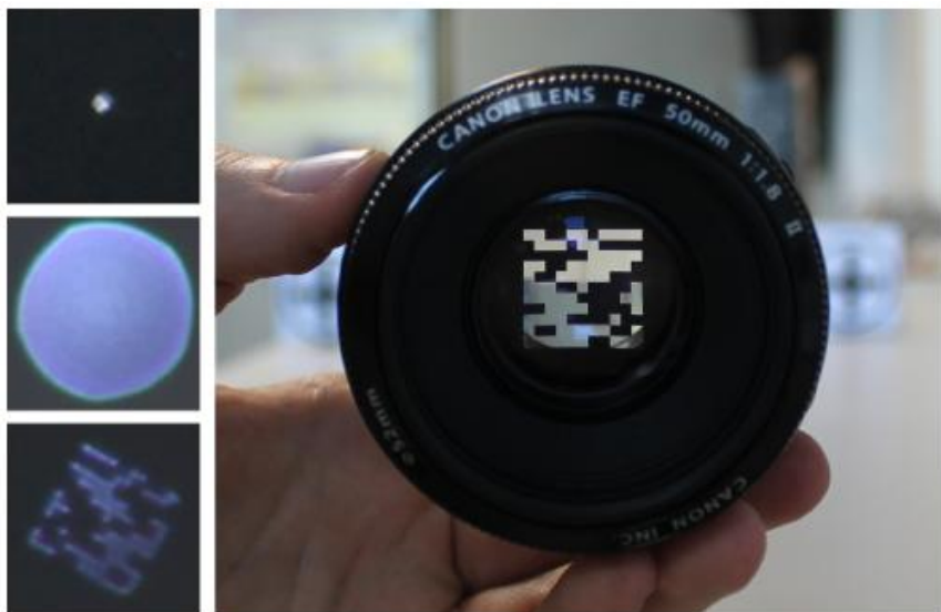
Figure 1: Left: Images of the response to a point light of different apertures (from top to bottom: focused aperture, defocused circular aperture -defocus depth = 90 cm- and one of our coded apertures -defocus depth = 90 cm-, shown in the right). A LED and black cardboard were used to create the point light. Right: Canon EF 50mm f/1.8 lens with one of our coded apertures.
