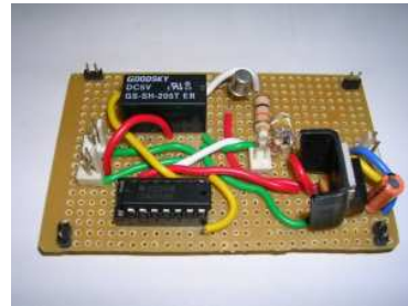
Figure 6: The Power Switching Circuit: Picture
