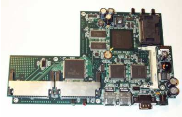
Figure 2: The Soekris net4521 single board computer
