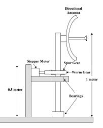
Figure 3.10: Mounting prototype
