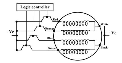
Figure 3.8: Stepper Motor circuit
