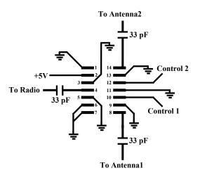
Figure 3.4: RF-Switch with RSW-2-25-P
