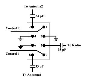
Figure 3.3: RF-Switch with PSW-1211
