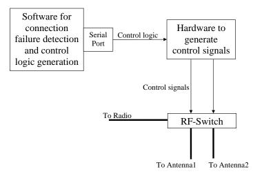
Figure 3.2: Block diagram of Replication solution
