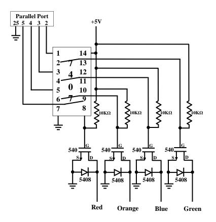
Figure 3.9: Circuit for stepper motor
