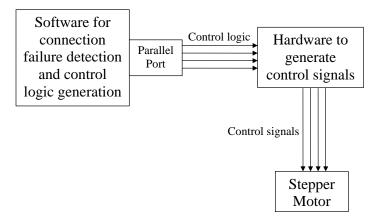
Figure 3.7: Block diagram of Replication solution
