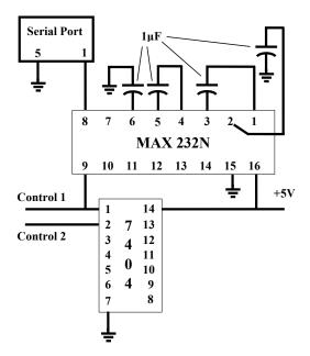
Figure 3.5: Hardware for generating control logic
