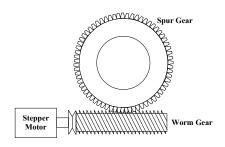
Figure 3.11: Spur Gear and Worm Gear
