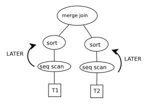
Figure 6: Asynchronous Iteration with Sort/Merge
