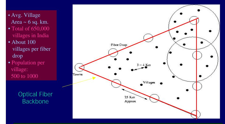
Domestically, 30,000 of BSNL's exchanges are connected by fiber an average of one exchange for 20 villages, not including the contribution of other operators. Thus, almost unlimited bandwidth is already possible.
