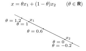
affine set: contains the line through any two distinct points in the set example: solution set of linear equations  $\{x \mid Ax = b\}$  in ear algebra and (conversely, every affine set can be expressed as solution set of system of linear equations)
