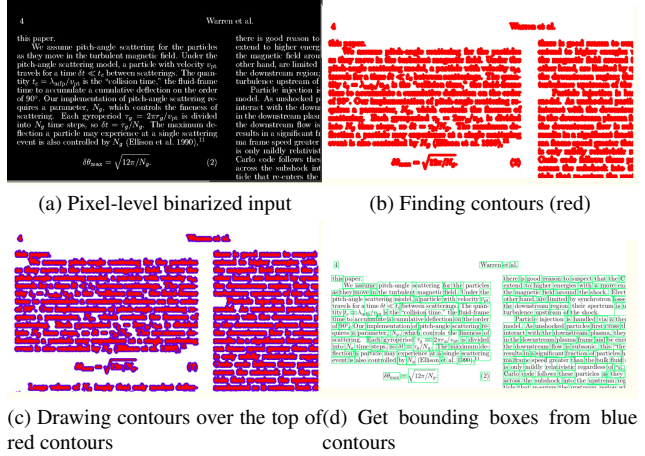
Figure 2. Workflow for Contour-based processing to get word level bounding boxes
