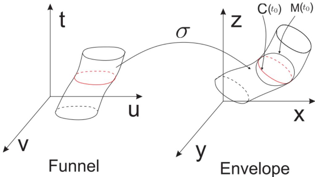
Figure:  $\sigma$  maps funnel ( $\mathcal{F}$ ) in param. space to envelope ( $\mathcal{E}$ ) in object space
