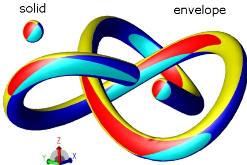
Figure: A solid swept along a trefoil knot.
