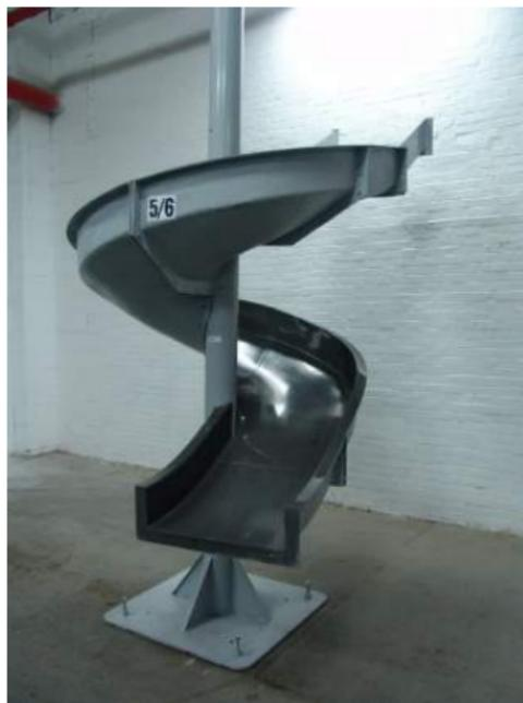
Figure: Gravity chute. Source: SigmaPackaging.com
