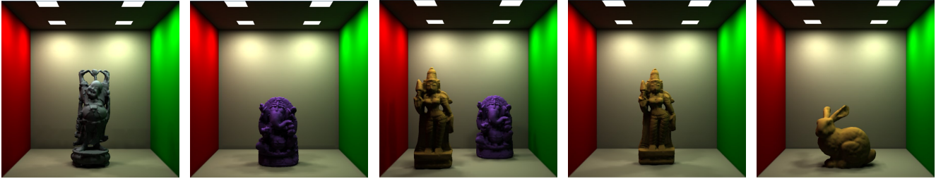
Figure 12. Point models rendered with diffuse global illumination effects of color bleeding and soft shadows. Pair-wise visibility information is essential in such cases. Note that the Cornell room as well as the models in it are input as point models.
