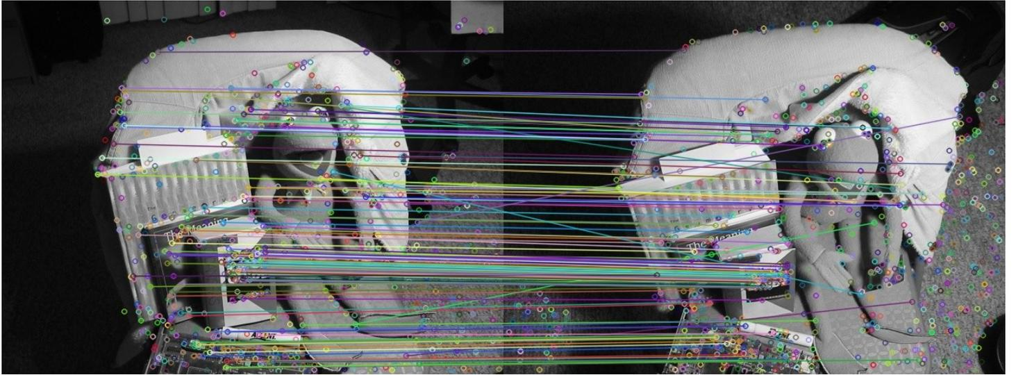
Figure 3.3: Point Correspondences using RANSAC and Five Point Algorithm on KERMIT data set
