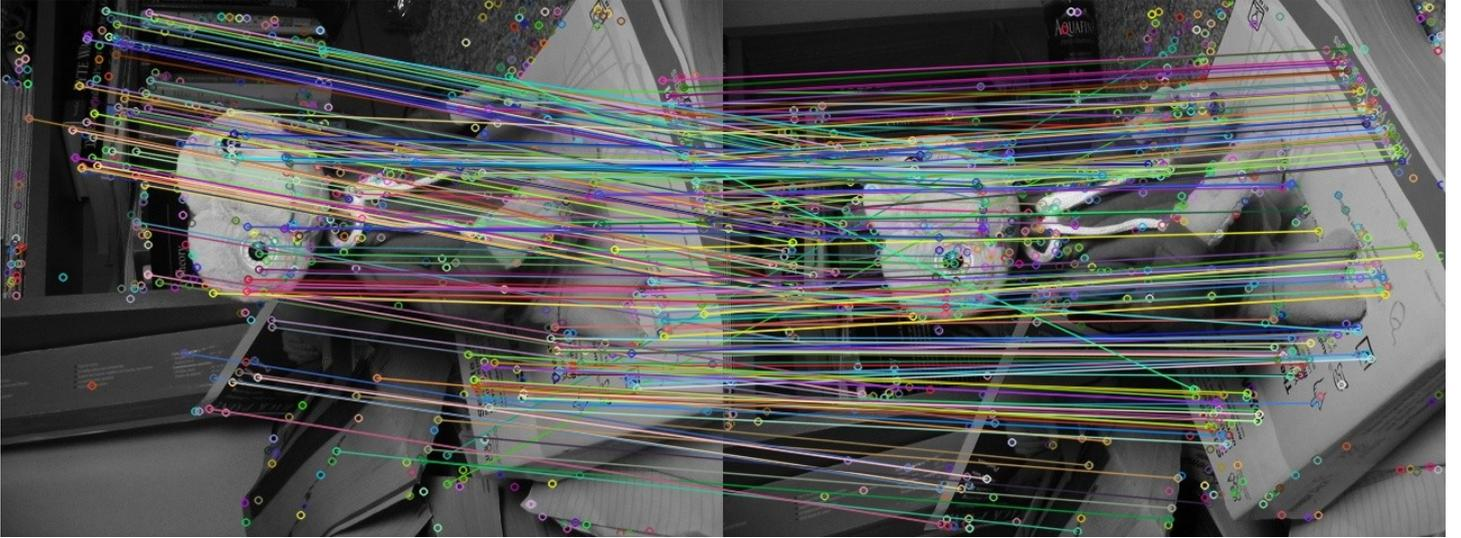
Figure 3.5: Point Correspondences using RANSAC and Eight Point Algorithm on ET data set
