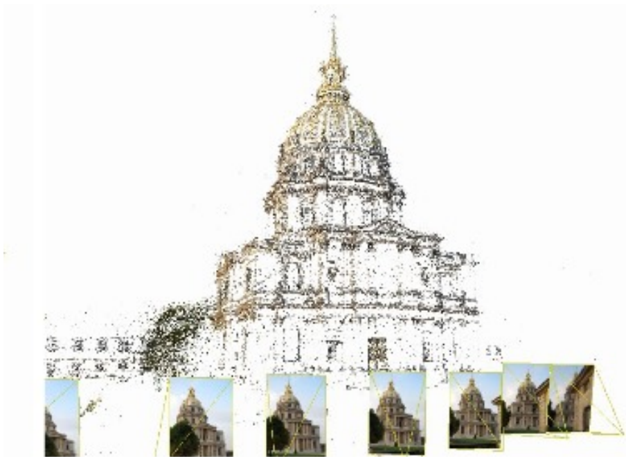
Figure 1.2: Shows a sparse and incomplete point cloud generated by SFM [1]
