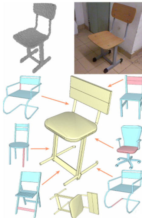
Figure 2.5: The above figure shows the final reconstructed model from scan data by parts borrowed from different repository models. Here the H shape base type example did not exist in the repository but recreated from other parts [3].
