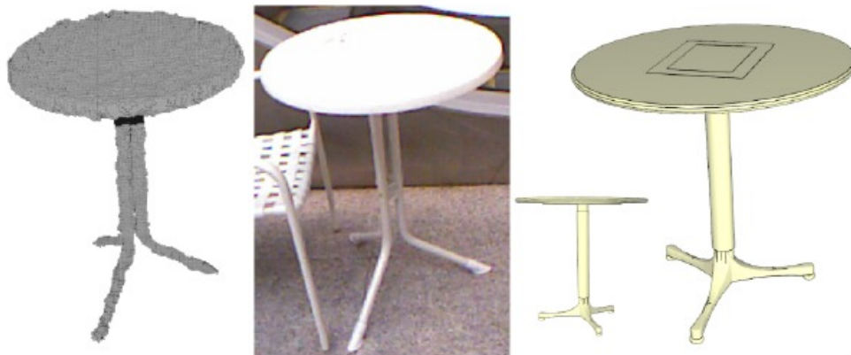
Figure 2.7: The above figure shows the failure of the part matching algorithm to discriminate between 3 slim pillars that are close to each other[3].
