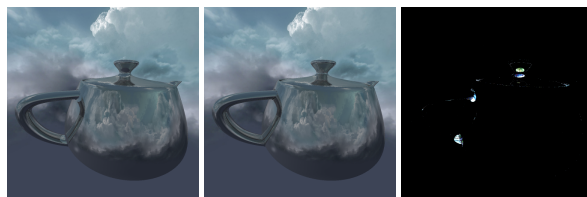
Figure 10: Regular ray tracing with secondary rays having multiple intersections with the same surface (left) vs. results from our system that avoids this issue for secondary rays (center), and 4X difference image between the two results (right).
