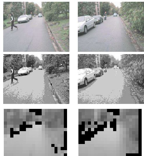
Figure 6: Some results of the SLOD: from top to bottom, the image at t (1 st column: image 5800, 2 nd column image 5870), the image at t after quantification (6 levels), and the ‘correspondent’ image LR after estimation of spatial translation of the image at t . The black pixels are the pixels of change or detected objects (except at the image border). Notice that even cars near the horizon and motorbike are well-detected.
