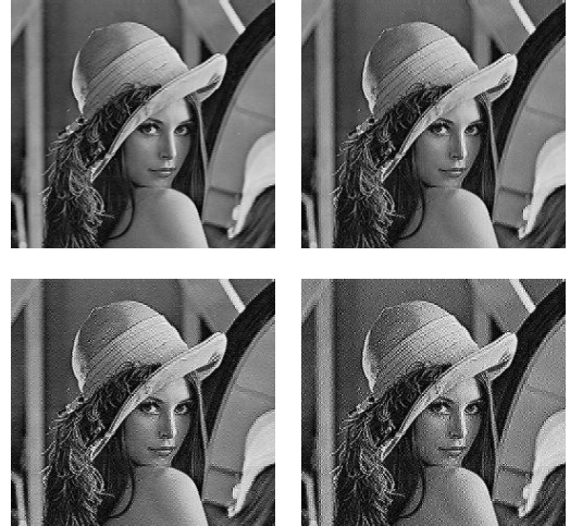
5: Watermarked copies of Lena image after multiple embedding a) single, b) twice, c) thrice, d) four times, without control distortion.
