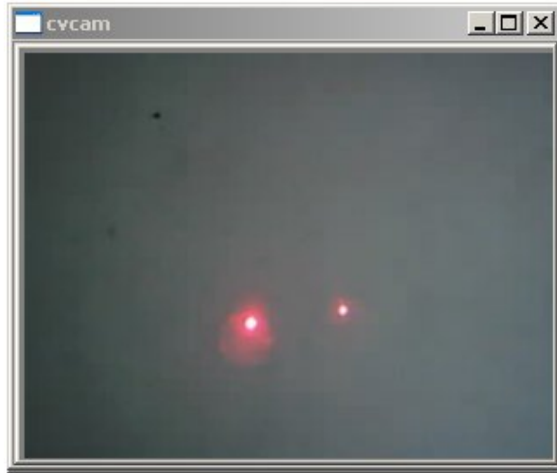
Figure 3. Multiple laser pointers captured by an inexpensive camera. Notice how a red laser pointer appears white due to saturation.
