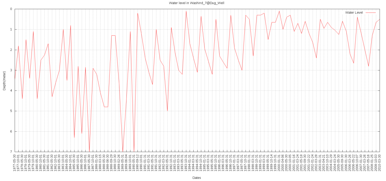
Figure 4.5: Water level in Washind_1_Dug_Well over the years.
