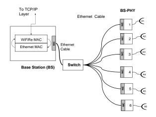
Fig. 6. BS hardware: proposed WiFiRe real system component
