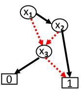
f = ite(x<sub>1</sub>, ite(x<sub>2</sub>, 1, ite(x<sub>3</sub>, 0, 1)), ite(x<sub>3</sub>, 0, 1))
