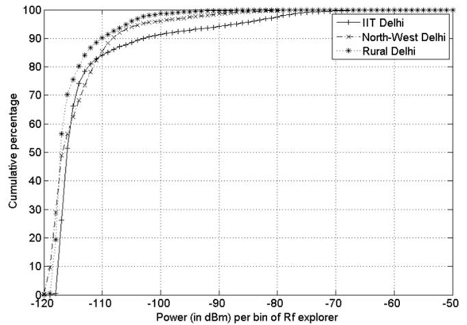
Fig. 6. Cumulative distribution of Power (240-960 MHz) for 24 hours
