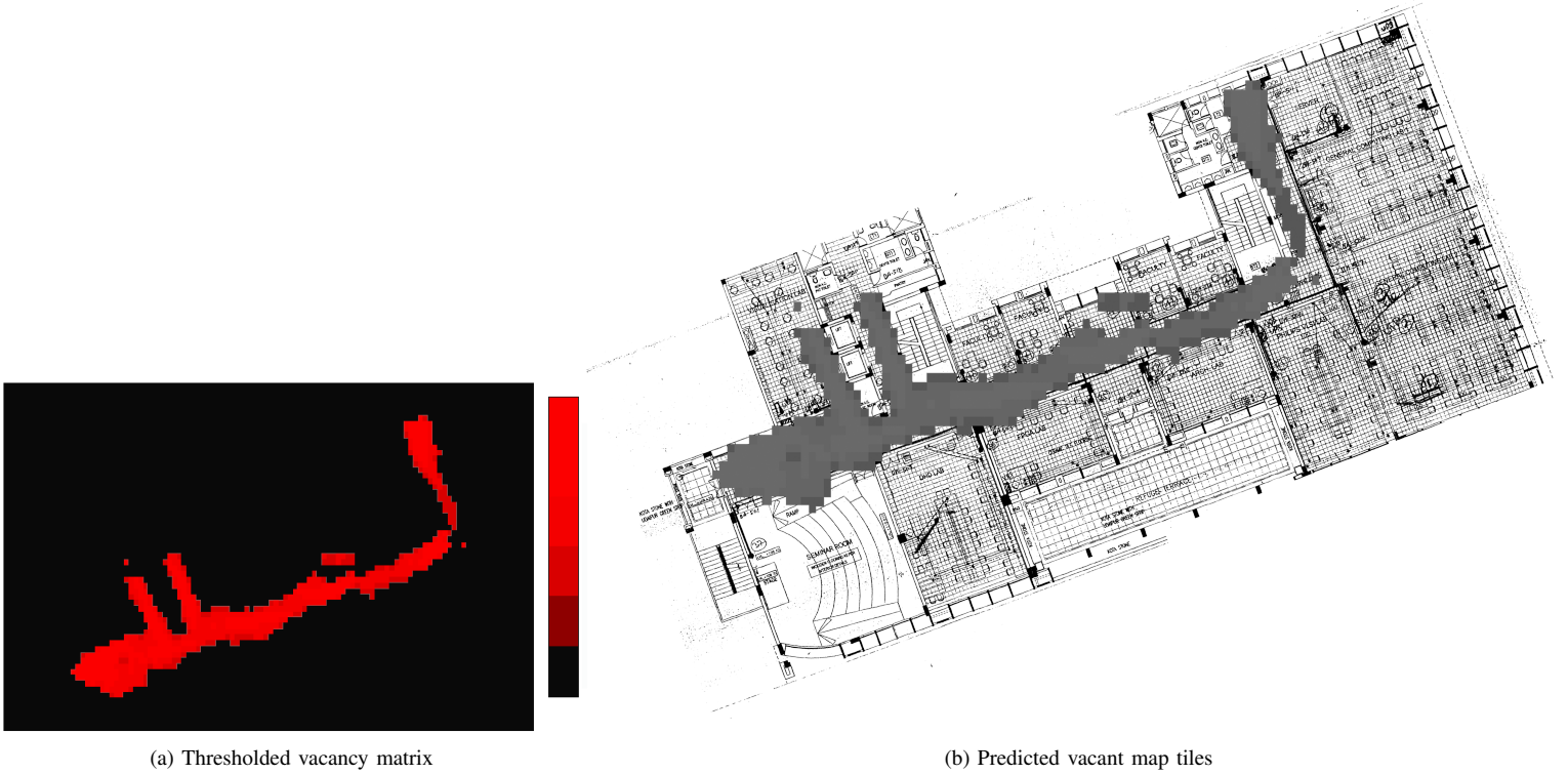
Fig. 7. (a) The thresholded vacancy matrix. The various colours in the heatmap are arranged in the colourbar, from bottom to top, in an increasing order of the sets of values that they represent. (b) The predicted vacant tiles are shaded in dark colours and overlaid over the reference floorplan.
