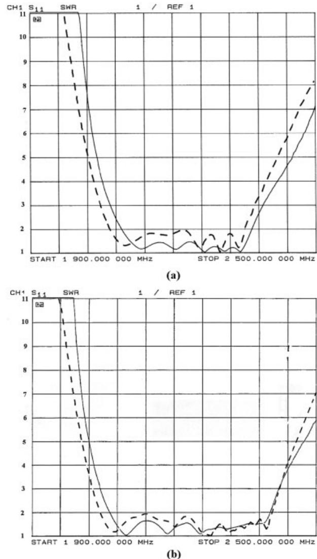
**Figure 5** Comparative plot for measured and simulated VSWR for (a) configuration with 11 strips; (b) configuration with 12 strips; (—) measured, (---) simulated
