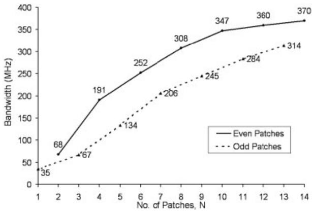
**Figure 4** Comparative plot for BW increment for configurations with even and odd number of patches
