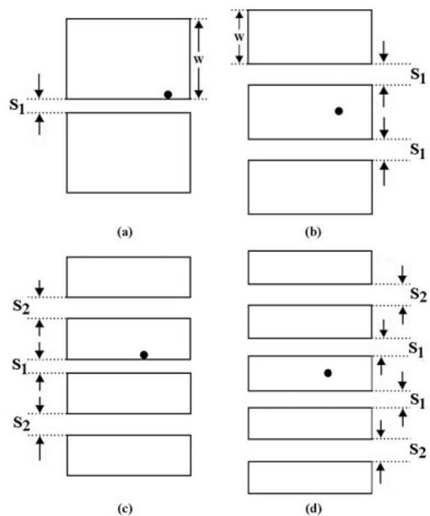
**Figure 1** Gap coupled configurations formed by splitting single RMSA into (a) two patch, (b) three patch, (c) four patch, and (d) five patch configurations
