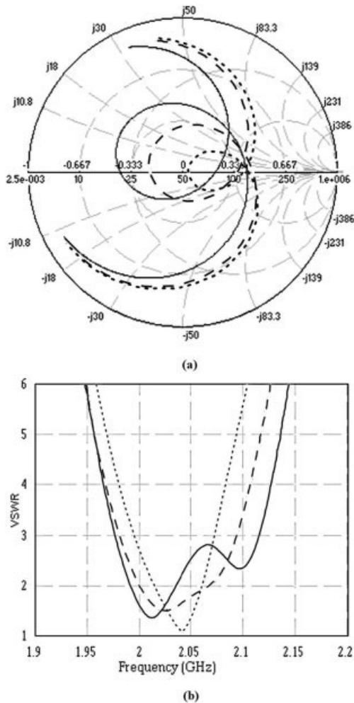
**Figure 2** Effect of gap on (a) input impedance loci, (b) BW for two patch configuration for three different gaps (—)  $S_1 = 1$  mm, (---)  $S_1 = 1.7$  mm, (.....)  $S_1 = 4$  mm
