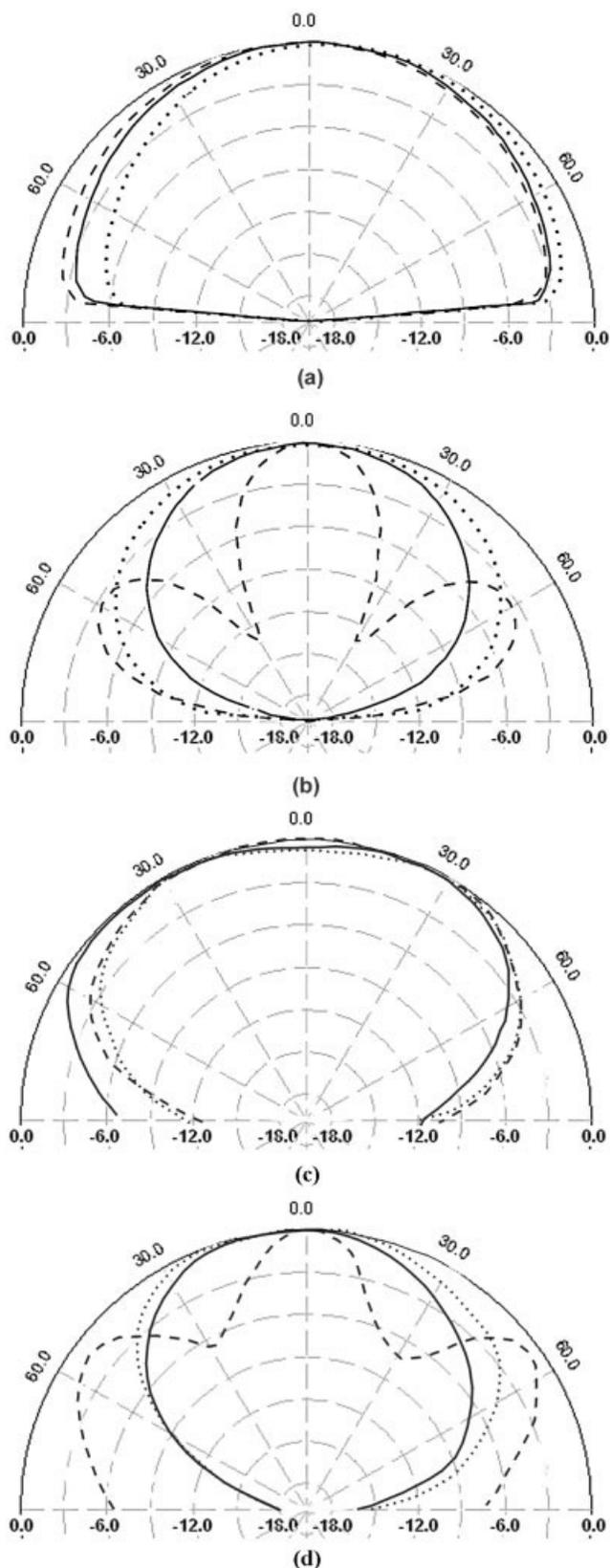
**Figure 6** Radiation pattern for 11 patch configuration at three different frequencies (—) lower band edge, (---) centre, (.....) upper band edge; simulated (a) E plane; (b) H plane, measured; (c) E plane; (d) H plane
