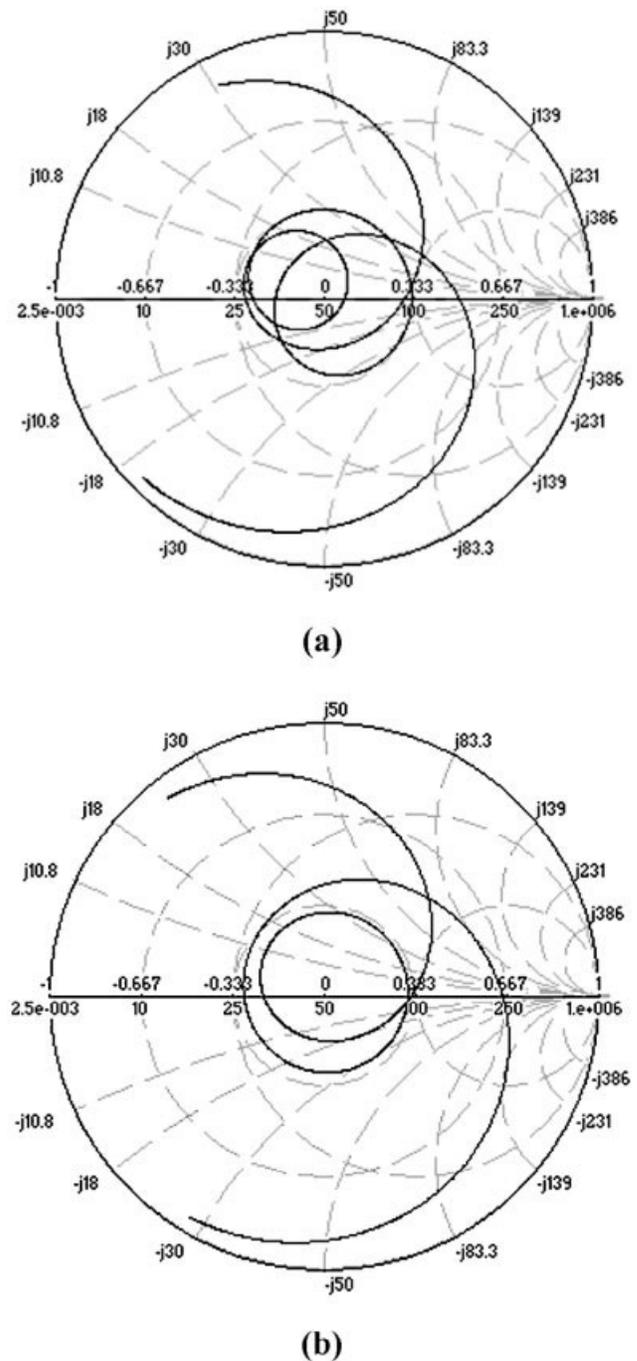
**Figure 3** Input impedance loci for (a) four patch configuration,  $S_1 = 1.7$  mm,  $S_2 = 2.8$  mm and (b) five patch configuration,  $S_1 = 3.2$  mm,  $S_2 = 6.5$  mm
