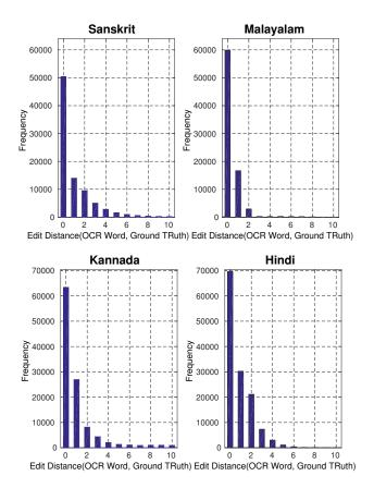
Fig. 3. Histogram of edit distance between OCR word and corresponding ground truth word pairs. As shown, most of the erroneous OCR words (with edit distance  $\geq$  1) exhibit confusion on one character and the frequency of erroneous words exponentially decreases with edit distance.
