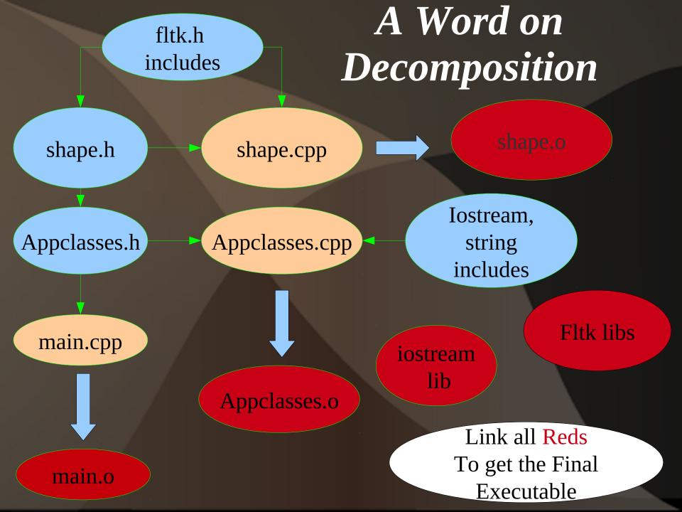
target: dependent1 dependent2 Command to generate or achieve the target dependent1: dependent3 dependent 4 Command to generate dependent1
