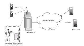
Figure 1. Typical mobile computing scenario
