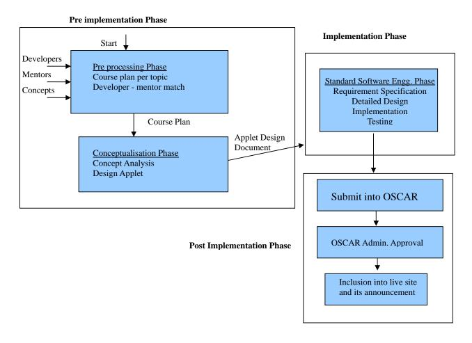
Fig.4: Applet development life cycle – A flowchart
