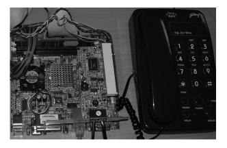
Fig. 4. Integrated exchange and gateway hardware
