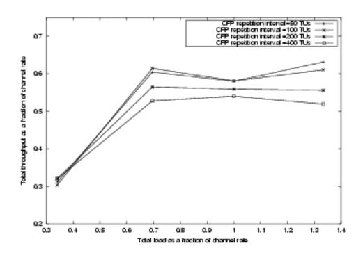
Figure 6.1: Throughput in PCF with PRRS for different CFP repetition interval with 32 active nodes
