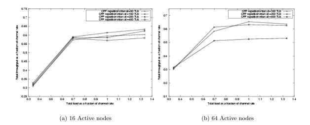
Figure 6.2: Throughput in PCF with PRRS for different CFP repetition interval with 8,16 and 64 active nodes.
