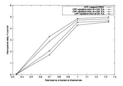
Figure 6.5: Delay characteristic of PCF with PRRS for different CFP repetition interval with CFP adaption enabled PCF with PRRS
