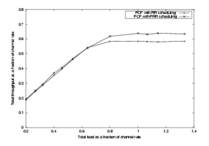
Figure 5.1: Throughput Comparison between PCF with PRRS and non optimized PCF with RRS. Total node =32 and 25% active node
