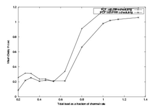
Figure 5.5: Average Delay comparison between PCF with PRRS and PCF with RRS. Total node =32 and 25% active node
