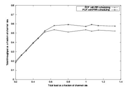
Figure 5.2: Throughput Comparison between PCF with PRRS and non optimized PCF with RRS. Total node =64 and 25% active node
