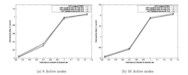
Figure 6.7: Delay characteristic of PCF with PRRS for different CFP repetition interval with CFP adaption enabled PCF with PRRS, having 8 and 16 active nodes.
