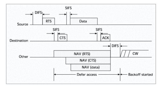
Figure 2.5: Transmission of an MPDU using RTS/CTS
