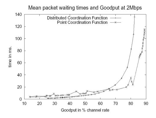
Figure 3.1: Comparison of mean packet waiting and goodput between DCF and PCF at 2 Mbps. 15 Nodes,1 PC and 1500 bytes packet size.
