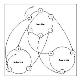
Figure 4.2: Example of stations/nodes in Active and Passive list. The order is imposed by the Node list.
