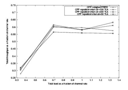
Figure 6.4: Throughput comparison of PCF with PRRS for different CFP repetition interval with CFP adaption enabled PCF with PRRS
