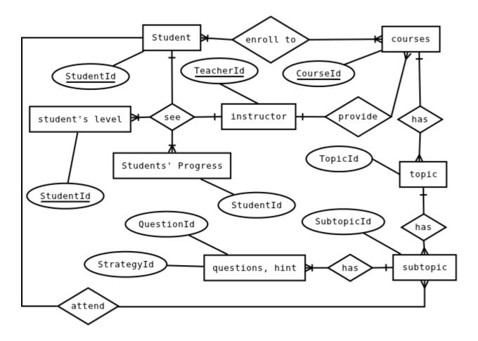
Figure 5.3: E-R Diagram of ITS with scaffolding.
