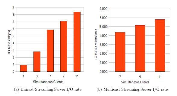
Figure 5.2: Comparison Of Unicast and Multicast Server I/O rate
