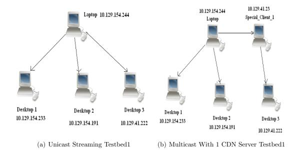
Figure 5.1: Testbed for Low scale Streaming Experiment
