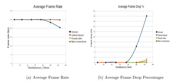
Figure 5.15: Comparison Of Average Frame rate and Average frame drop
