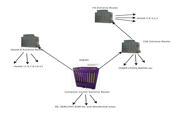
Figure 3.2: Part Of IITB Network Physical Diagram.
