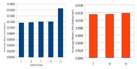
(a) Unicast Streaming Clients average mean (b) Multicast Streaming Clients Average mean packet delay
