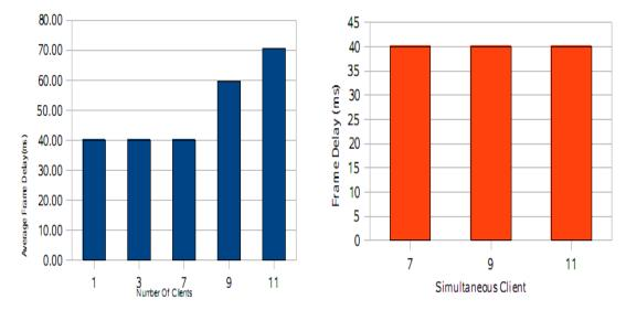
(a) Unicast Streaming Client Average Frame (b) Multicast Streaming Client Average Frame Delay Delay
