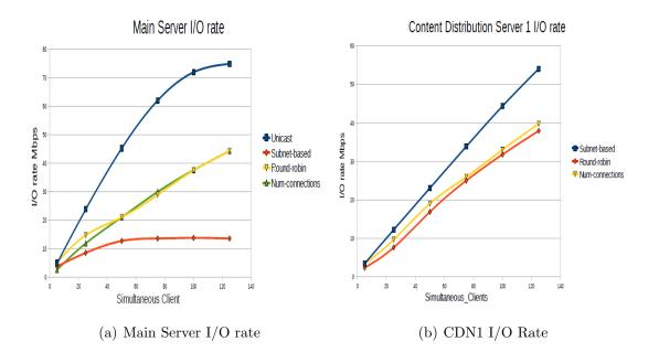
Figure 5.17: I/O rate of Main Streaming Server and CDN Server1
