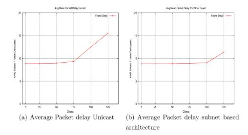
Figure 5.14: Comparison of clients avg-packet-delay for Unicast architecture and CDN Subnet based redirection algorithm
