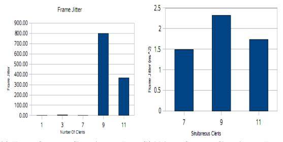
(a) Unicast Streaming Client Average Frame (b) Multicast Streaming Client Average Frame Jitter
