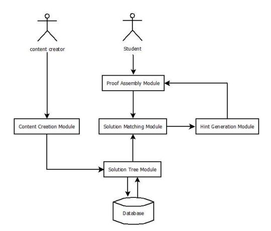
Figure 4.1: Workflow of the system showing all the modules
