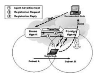
Figure 2.1: Working of Mobile IP
