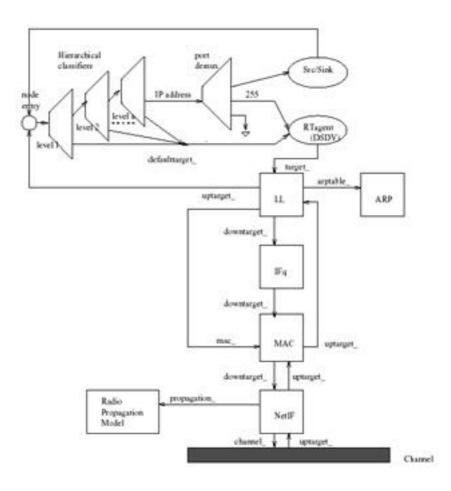
Figure 6.1: Node Architecture in Mobile IP
