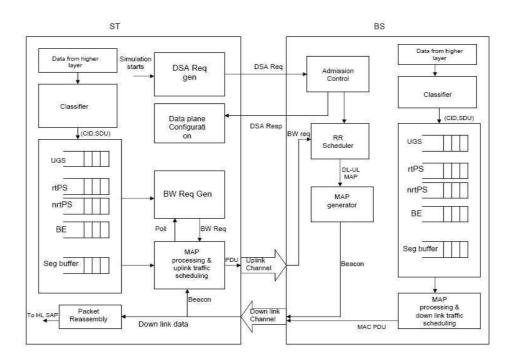
Figure 4.1: WiFiRe Model design block diagram
