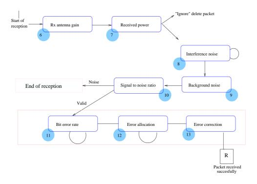
Figure 4.7: Receiver pipeline stages
