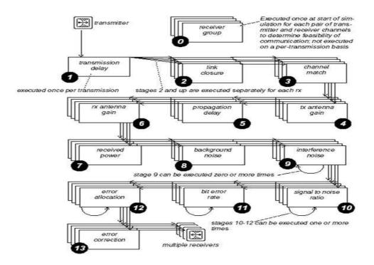
Figure 2.3: Radio Transceiver Pipeline Execution Sequence [7]
