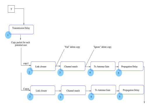
Figure 4.6: Transmitter pipeline stages
