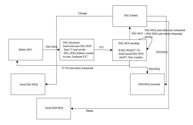
Figure 3.11: Remotely initiated DSC
