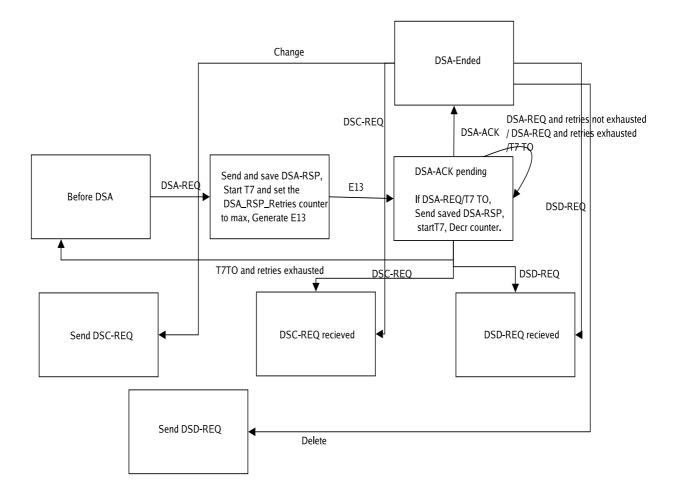
Figure 3.9: Remotely initiated DSA
