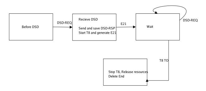
Figure 3.12: Remotely initiated DSD
