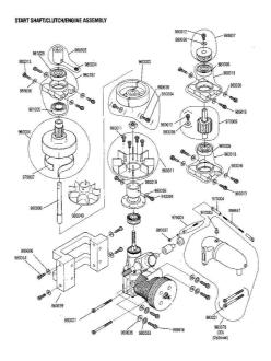
Figure 2.6: Objects in a Ergo 30/46 CCPM radio control helicopter assembly
