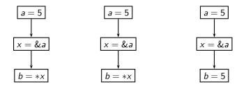
Original Program Constant Propagation Constant Propagation without aliasing with aliasing
