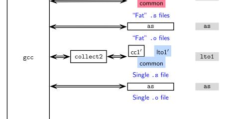
The GNU Tool Chain for Non-Partitioned LTO Support
