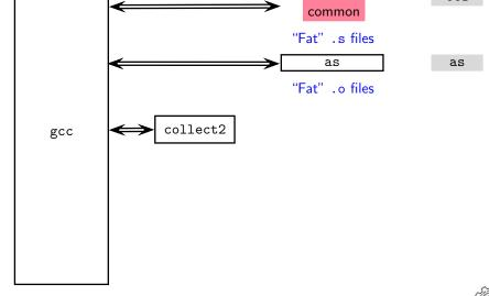
The GNU Tool Chain for Non-Partitioned LTO Support
