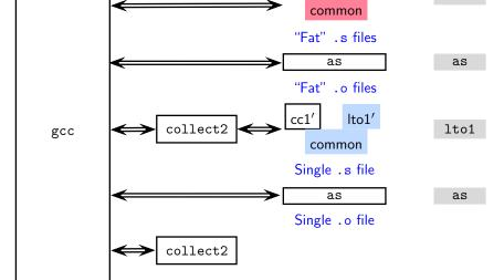
The GNU Tool Chain for Non-Partitioned LTO Support
