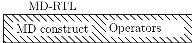
Figure 5.1: The MD-RTL language. The MD constructs describe properties of target instructions and the operators (of the fictitious processor) capture the target instruction semantics.
