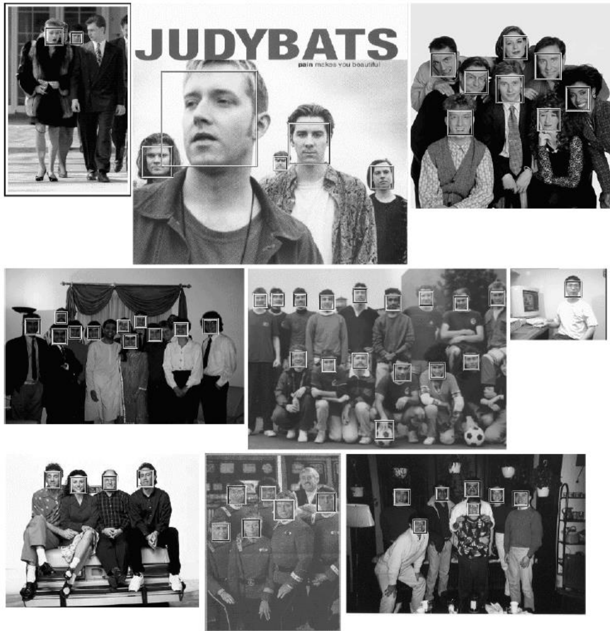
Figure 10: Output of our face detector on a number of test images from the MIT+CMU test set.
