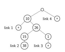
The IP address of a packet is matched with the trie. The link with the longest match will receive the packet.
