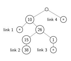
We match the IP address of a packet with the trie. The link with the longest match receives the packet.
